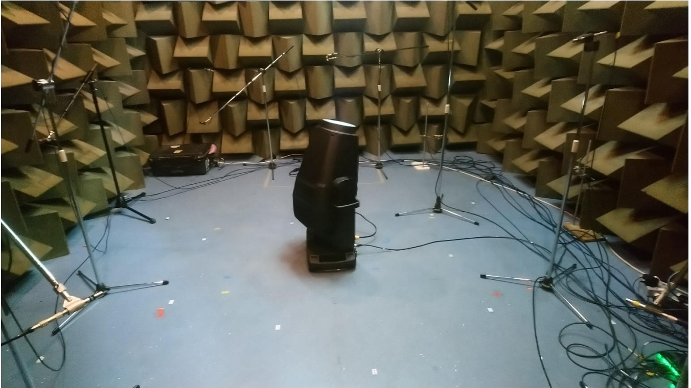
Figure 2.1 – Example of the typical arrangement of a unit under test, as mounted in the hemi-anechoic chamber at the University of Salford. (N.B. this image does not represent the specific unit covered by this Test Report.)
