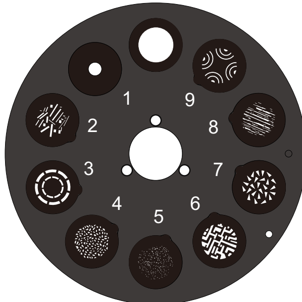
Gobo Wheel 2 Static gobo wheel
